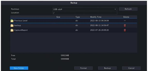
6. Select the partition and storage path, click Backup. Then the recordings are saved to the specified path on the storage device. You can also create a new folder for the recording(s) by clicking New Folder.
