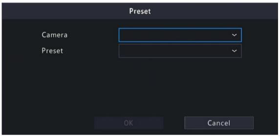
2. Select the camera to perform this action and select the preset you want the camera to go to when an alarm
