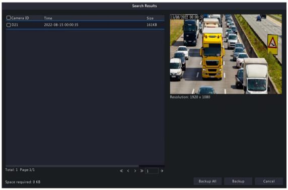
**Note:** The image resolution depends on the resolution from the output interface and the number of windows displayed when the snapshot is taken.
