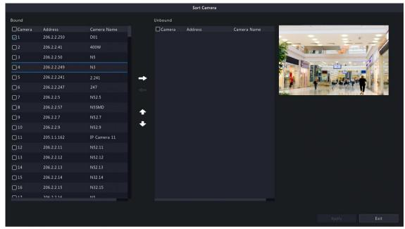
2. In the left list, select the check box for camera 1 and click \_\_\_\_. Then camera 1 with IP 206.2.2.250 now appears in the right list. Perform the same operations to camera 4.
