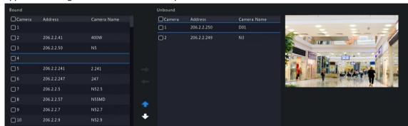
3. In the right list, select the camera 4 with IP 206.2.2.249 and click \_\_\_\_. Then camera 4 appears at the previous line of camera 1 in the list. Perform the same operations to camera 1, so camera 1 appears at the previous line of camera 4 in the list.
