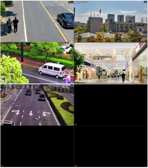
• When Max. Alarm-Triggered Live View Windows is set to 9 Windows, the live view page plays the live video of each camera in 9-split mode. If more than 9 cameras are linked, the live video switches at 5s.
